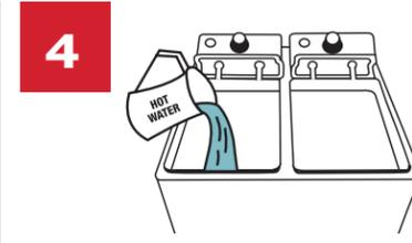
Add hot water to completely fill the fryer well. Set the thermostat to 200°F/93°C. Turn on the fryer and run it for 1–2 hours until clean.
